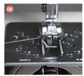
back to its regular position on the left, then snip the thread joining it to the spool and remove the bobbin.
